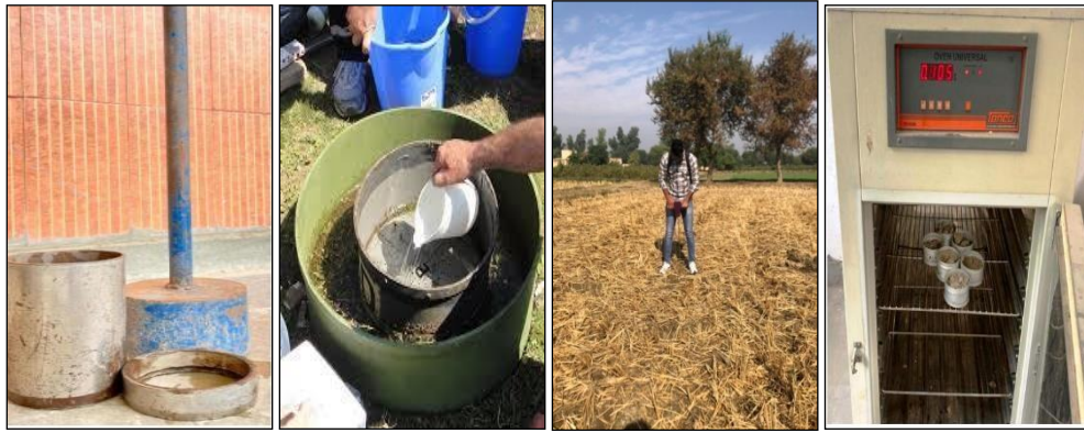
Figure.2. Measurement of Soil bulk density, moisture content, soil cone index and water infiltration rate
